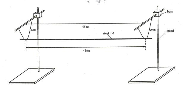
The two boss rods should be parallel, equal in heights above the bench and 45 cm apart. The two strings supporting the steel rod should be 45 cm apart.
