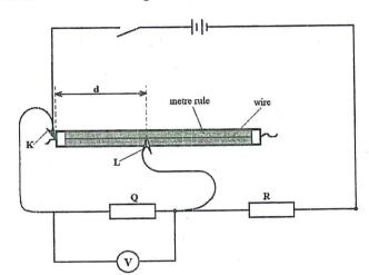
Place L at a length  $d = 20 \, cm$ , keep the length constant through throughout the experiment. The distance between K and L is d as shown above. Close the switch and record the voltmeter reading V.
