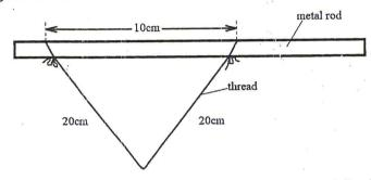
Each side of the loop on the rod should be approximately 20 cm long.
