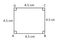
Draw line AB, 4.5 cm long1 markConstruct a 90° at point A towards D1 markMeasure and mark 4.5 cm at point D1 markFrom point B and radius 4.5 cm draw and arc above1/2 markFrom point D and radius 4.5 cm draw and arc horizontally to get point C 1/2 markABCD is the complete square.
